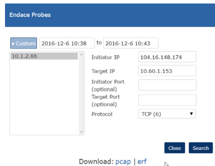
Figure 2. Search parameters are pre-filled, searching returns a packet capture file of related packets
