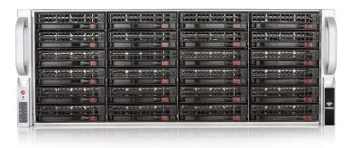
EndaceProbe™ 9200 G4 Series Analytics Platforms are ultra high-capacity, high-performance appliances capable of providing 100% accurate network history recording and Playback on up to eight 1/10GbE or two 40GbE links.
